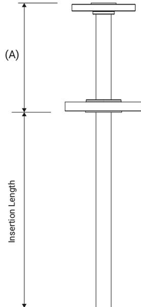
The CFI Series non-retractable injection quills are selected based on their ability to handle high-pressure and/or high-temperature applications where threaded connections are not permitted. They are also common in applications that require the rigid integrity of a non-retractable is needed to stand up against excessive turbulence or other adverse process flow conditions.
