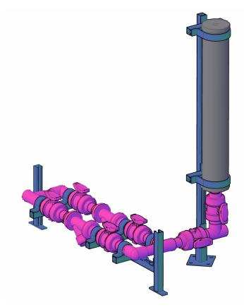
We know it is not always practical to fit larger calibration columns into a dosing skid. To overcome this, we have developed a modular design piping and support system that we can supply as a complement to our 10L and 20L calibration columns.
