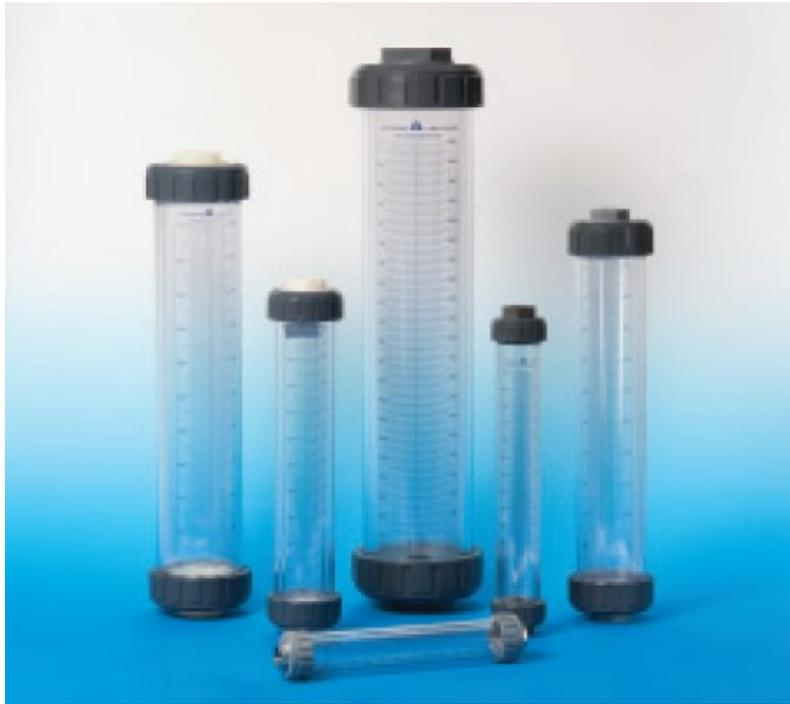
*Calibration Columns allow quick measurement to ensure accurate flow rates. Used when commissioning, maintaining pumps and checking processes.*
