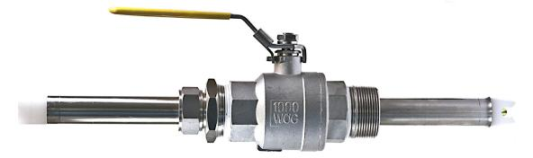
The LiveTap<sup>™</sup> Insertion Assembly is ideal for use in areas where down time is critical by allowing removal of the electrode from a live line or tank without process interuption. Fitted with a 1.5" ball valve, the pH or ORP electrode can be removed for maintenance by sliding the 316L Stainless Steel sheath through the valve and closing it off. Your unit is now safe to remove.
